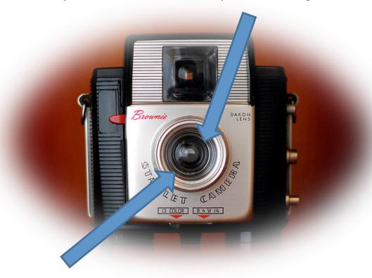
Example: When you take a picture, the *shutter* opens and lets light into the camera, allowing the film to capture the image.
