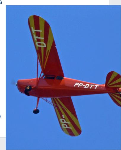
A plane's wings and tail are modeled after a bird, too. These structures are attached to the fuselage, just as a bird's wings and tail are attached to its body. The wings of a plane function like the wings of a bird, helping to lift the plane into the air. The tail of a plane also works like a bird's tail. It helps to stabilize
